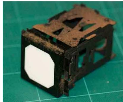
4. Remove main projection lens and replace with a tube of black paper or construct a box of black cardboard. (auto-focus mechanisms may need to be removed)
